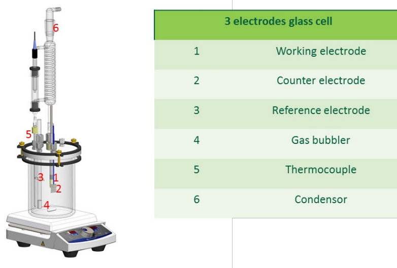
Figure 4. Configuration of the 3-electrode glass cell (figure courtesy of Cody Shafer)
